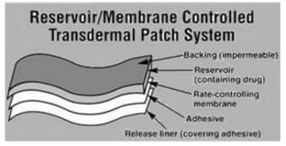
Fig. 3. Reservoir controlled transdermal patch system
