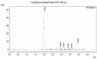
Fig. 2. Chromatogram of Atorvastatin calcium
