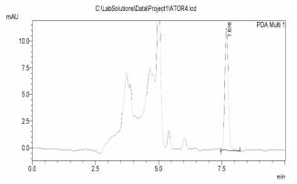
Fig. 5. Basic degradation of atorvastatin calcium
