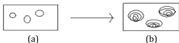
Fig. 1. Swelling mechanism of superdisintegrants a) Granules with superdisintegrants in aqueous media; b) Swelling of granules due to superdisintegrants
